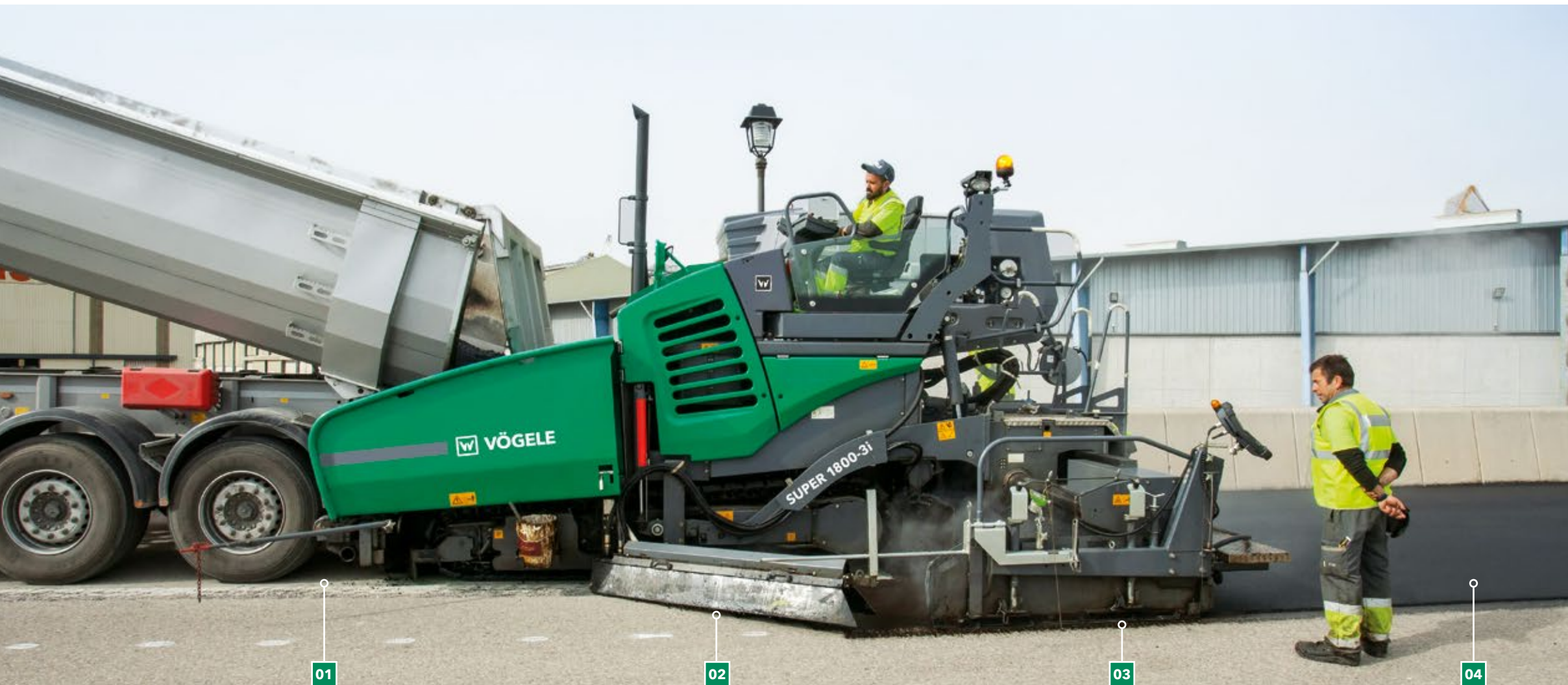
02 Hot bitumen emulsion at a temperature between 158 to 176 °F (70 to 80 °C) is applied by the spray paver.
