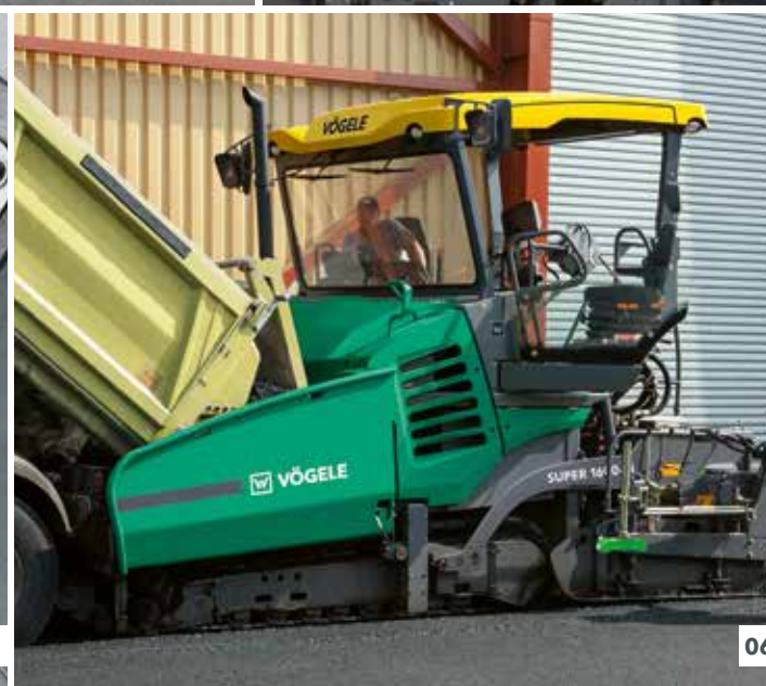
04 The paver operator's platform ensures maximum visibility. 05 Automated processes with AutoSet Plus. 06 PaveDock spring push-rollers and PaveDock Assistant communication system facilitate optimum feeding with mix.
